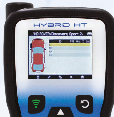
Start with the LF (left front) tyre
