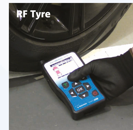
Repeat for the RF (right front) tyre
